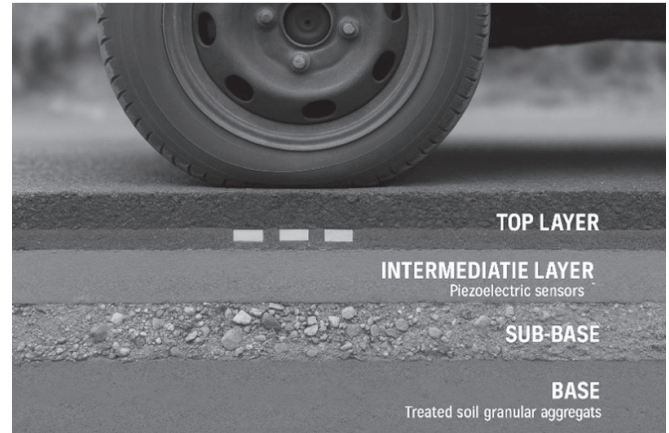
Figure 4. The layered structure of the piezoelectric pavement.
