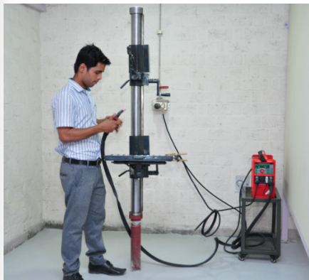
Trans-TIG Welding Station
