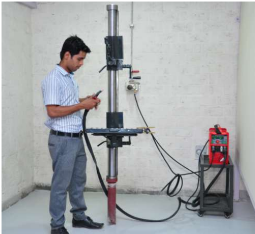
Trans-TIG Welding Station
