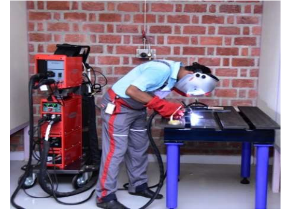
Magic Wave Welding Station
