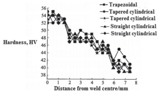
Figure 5. Micro hardness profile for various tool geometry [8].
