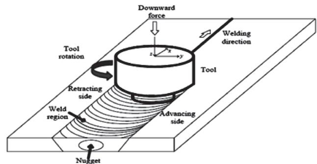
Figure 1. Schematic drawing of friction stir welding.
