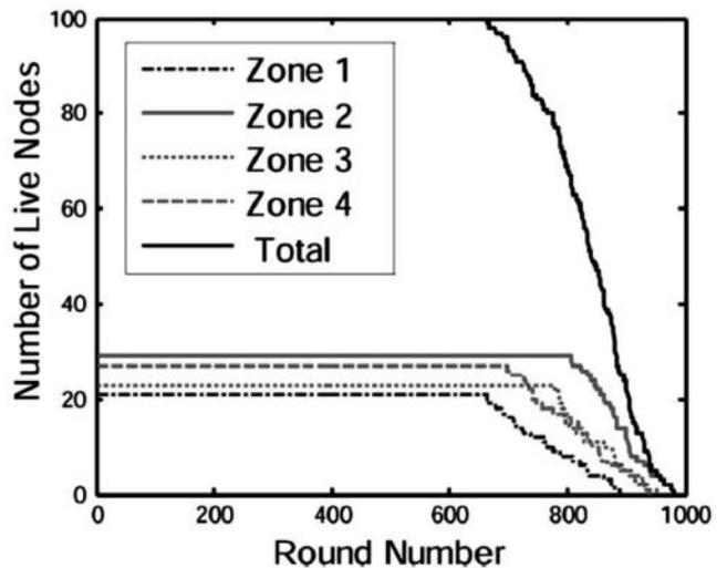
Figure 6. Performance (number of live nodes versus round) after introducing the DFS into the rectangular sensor area.
