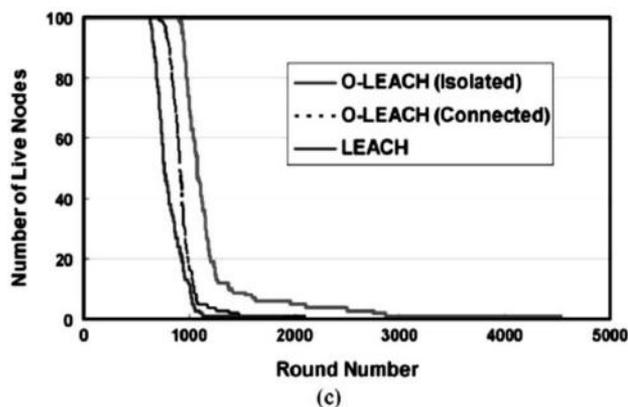
Figure 3. Simulation results of network performance in terms of lifetime (round number) using O-LEACH protocol. (a) Two WSNs can communicate with each other. (b) Two WSNs are isolated. (c) Typical lifetime evolution curves.
