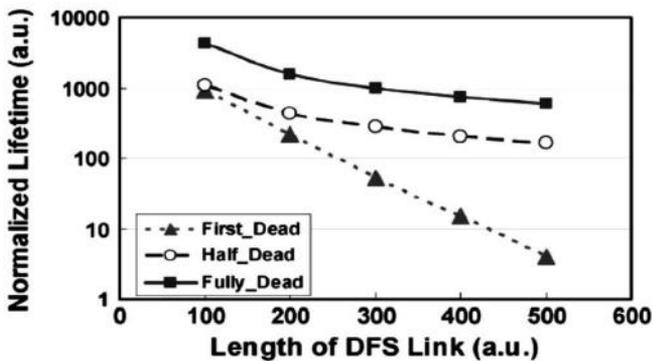
Figure 4. Normalized lifetime as we increase the length of DFS link (number of WSN nodes are increased proportionally, the widths of the DFS coverage area and the whole sensor field are fixed).
