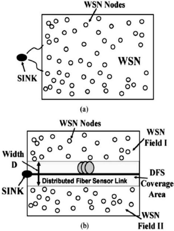
Figure 1. (a) Illustration of a WSN with randomly scattered nodes (sink node: no Energy restriction; WSN nodes: with energy restriction); (b) Sensor field consisting of a DFS link and two WSN fields (I and II), the sink node is located at one end of the DFS and the width of the DFS coverage area is  $D$ .
