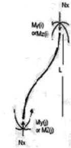
Figure 2. Beam-column with end moments.
