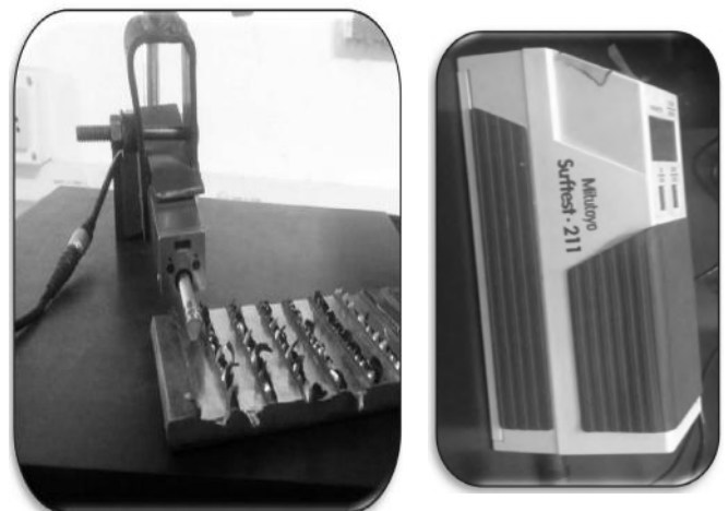
Figure 2. Measurement of surface roughness using Surf Test-211 series (Mitutoyo).
