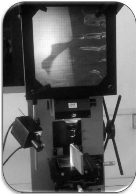
Figure 3. Profile projector for measuring burr size.
